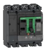
Circuit breaker, ComPacT NSX100B, 25kA/415VAC, 4 poles 4D (neutral fully protected), TMD trip unit 80A
